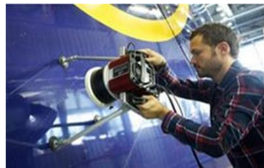
Figure 11 – The device of the active temperature method for the study of airplanes (Automation Technology, Germany) [2]
